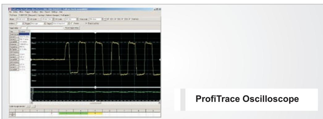
**P**rofiTrace is a PROFIBUS analyser which runs on ProfiCore USB hardware. The hardware and software package can be used to analyse the signal quality, and for bus monitoring, topology scan, reporting and master activities.
