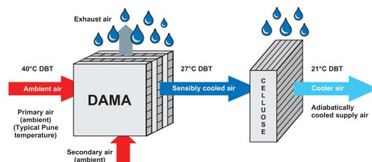
The primary air stream is cooled first with indirect evaporative cooling and then cooled further with direct evaporative cooling. The combination of these two stages results in improved cooling, taking the primary air temperature well below the concurrent ambient Wet Bulb Temperature.
